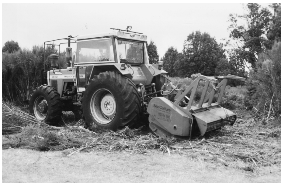
Figure 2. Picture of tractor and mulcher attachment used during the broom control demonstration trial.
